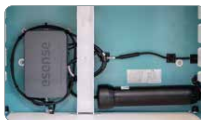
Non-visible battery kit located in the "crawl space" of the cart to optimize space and protect the kit from external impact.
